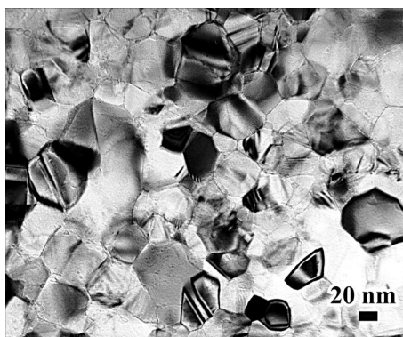
FIG. 1. Plan-view TEM micrograph of a typical TiO 2 film.
